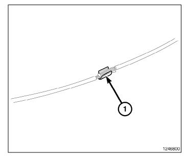
12. Place the strands of the power side wires overlapping each other inside of the splice clip (1).
